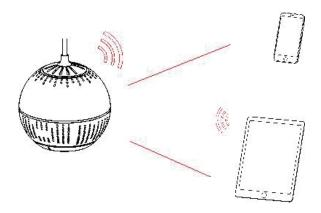
Wi-Fi STA Mode: Acting as terminal device, the lamp is connected to the home router, which is in the same network like the cellphone, and you can use the cellphone to control the lamp. This mode is applicable to synchronous control of multiple lamps.
