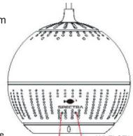
Wi-Fi AP mode switch hole (Use needle to poke it and keep pressing for 3 seconds to be in AP mode)
